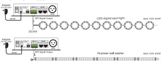
3. Connected with DMX 512 computer console to realize DMX decoder functions.
