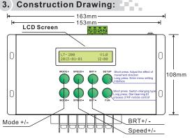
\*Long press Mode + to enter black change mode realizing power off, Long press Mode - to enter automatic change Mode 31.
