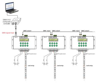
4. Connected with DMX 512 computer console, use the console to manage the controller
